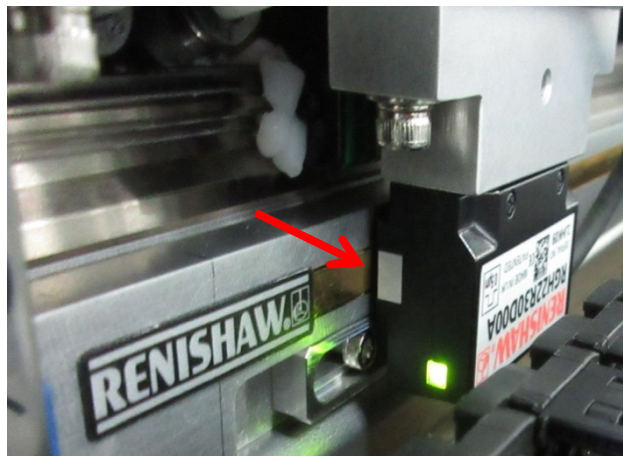
(b) Renishaw encoder gap is 0.8 \pm 0.15 \text{ mm}
