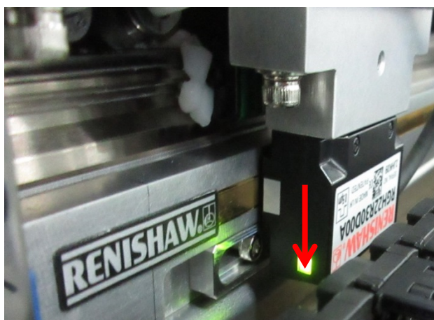
(c) Blue spacer attached with read head
