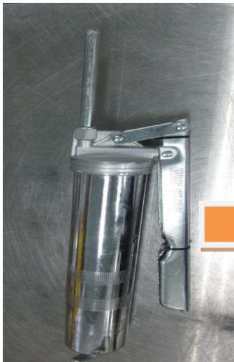
(a) Fill-in the grease
