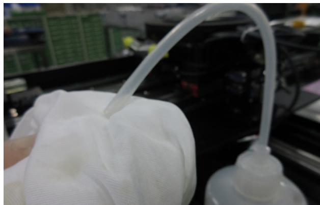
(b) Clean with wiper and Ethanol
